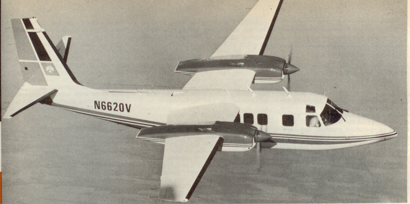
North American Rockwell's 685 is a pleasure to "drive" and ride, says author. Low noise level is impressive, as is cruise speed, which was clocked at 262 mph true airspeed, 7 mph higher than that stated in the aircraft's performance table.
